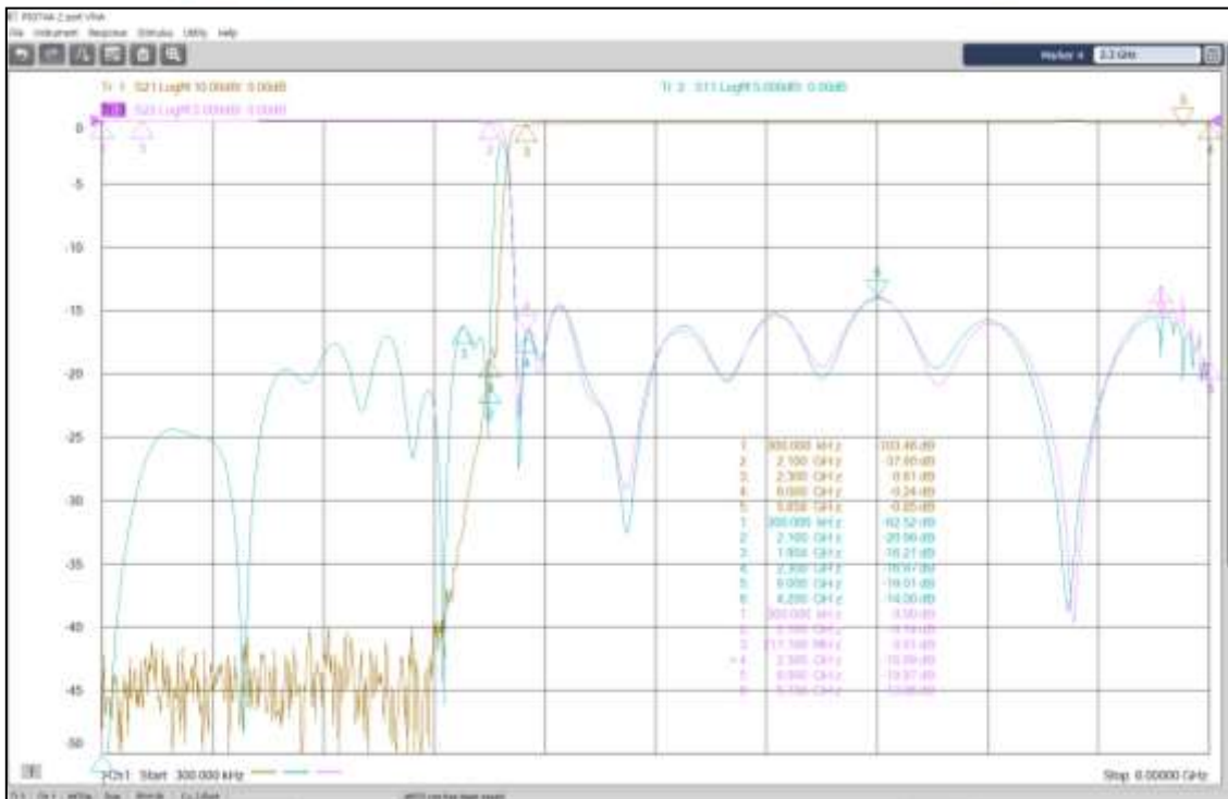
Diplexer CH2 path Transmission
